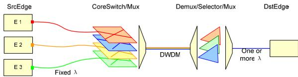
Figure 3 Two-layer network architecture
