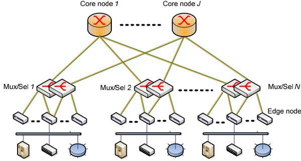
Figure 1 AAPN network model: three-layer overlaid tree topology
