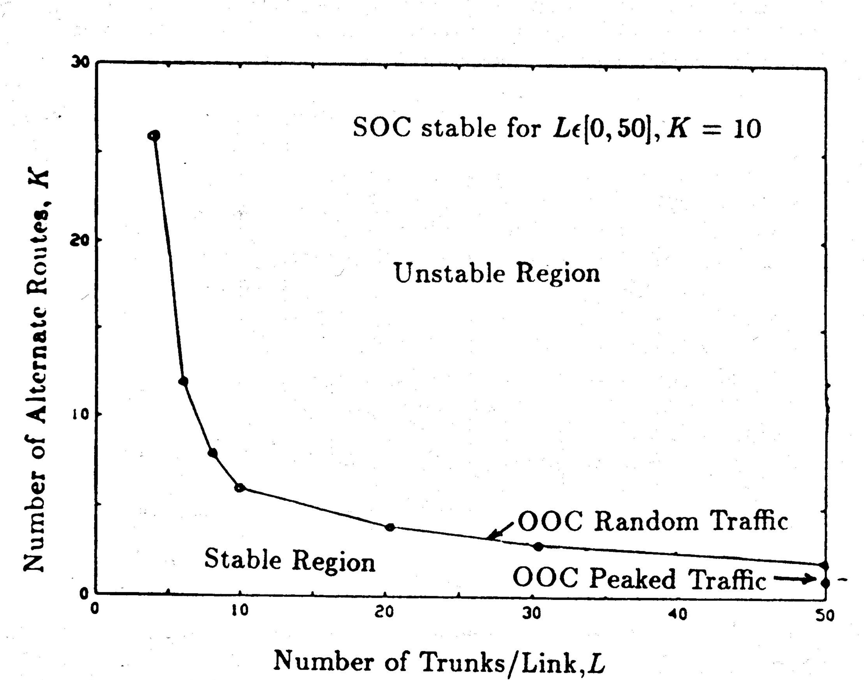
Figure 2. Uniform Finite Network Stability Boundary
