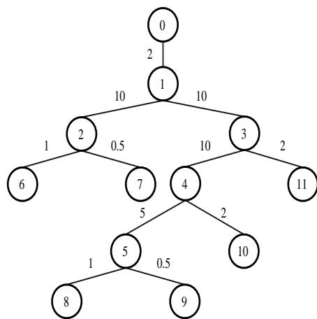
Figure 8: Tree-structured network topology used for ns simulation experiments. Source (node 0) transmits to 6 receivers (nodes 6-11). Link speeds in Mb/s are shown next to the links. Link  $i$  connects node  $i$  to its parent node  $\omega(i)$ , e.g. link 9 connects nodes 5 and 9.
