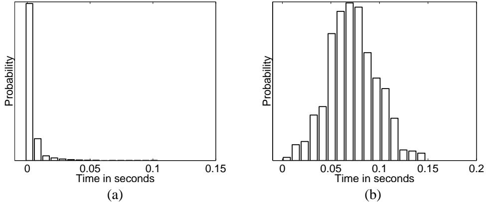
Figure 2: Delay histograms from two different Internet measurement sessions. 1000 measurements were made using the *netdyn* tool [2].
