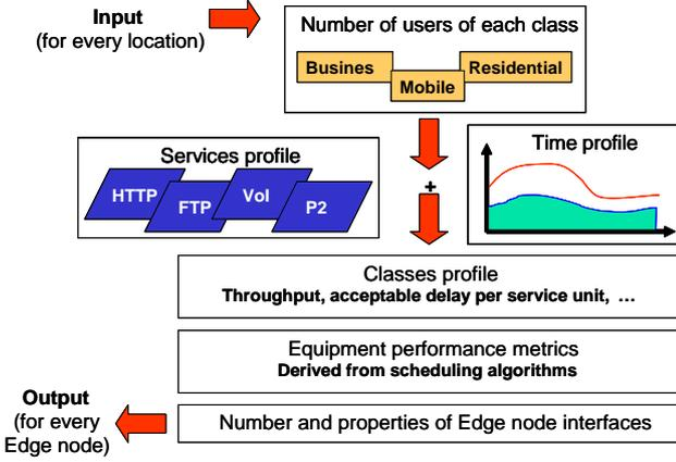
FIG. 2. WORKING PROCEDURE OF NETWORK DIMENSIONING
