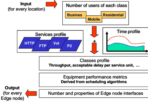
FIG. 2. WORKING PROCEDURE OF NETWORK DIMENSIONING
