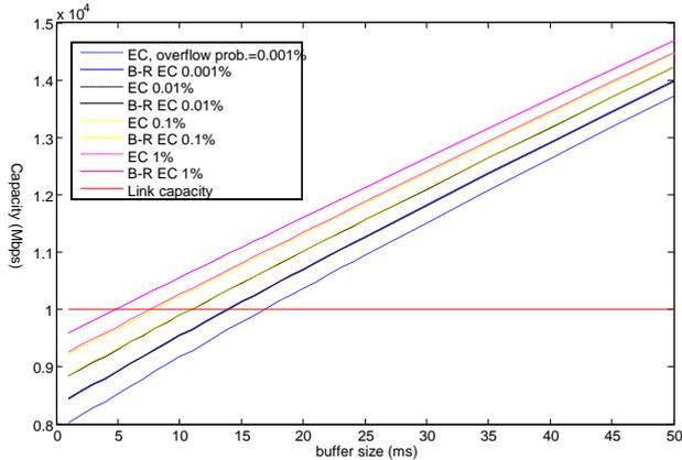
FIG. 3. EFFECTIVE CAPACITY WITH DIFFERENT OVERFLOW PROBABILITIES
