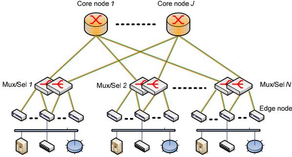
Figure 1 AAPN network model: three-layer overlaid tree topology
