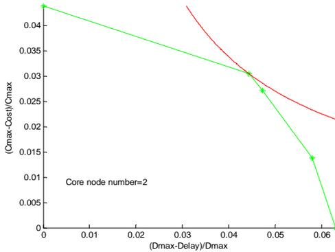
Figure 4 Pareto Boundary of delay vs. cost (2 cores)
