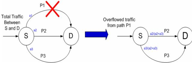
Fig. 5. An illustration of the routing algorithm
