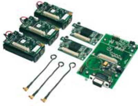
Fig. 2.3 Crossbow's MICA2 basic sensor network kit. This kit contains three MICA2 Processor/Radio Boards (motes), two MTS300 Sensor Boards (Light, Temperature, Acoustic, and Sounder), and one MIB510 Programming and Serial Interface Board (base station). Source: Crossbow ( http://www.xbow.com )
